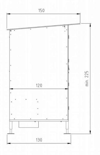
**Location Requirements:** A minimum distance of 50 cm must be maintained at the rear of the toilet cabin to ensure sufficient space for changing the feces containers.
